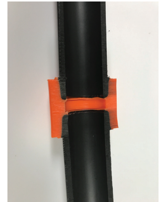
Inside cross section of socket fusion.
