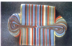
Cross section view of butt fusion melt pattern with bead.
